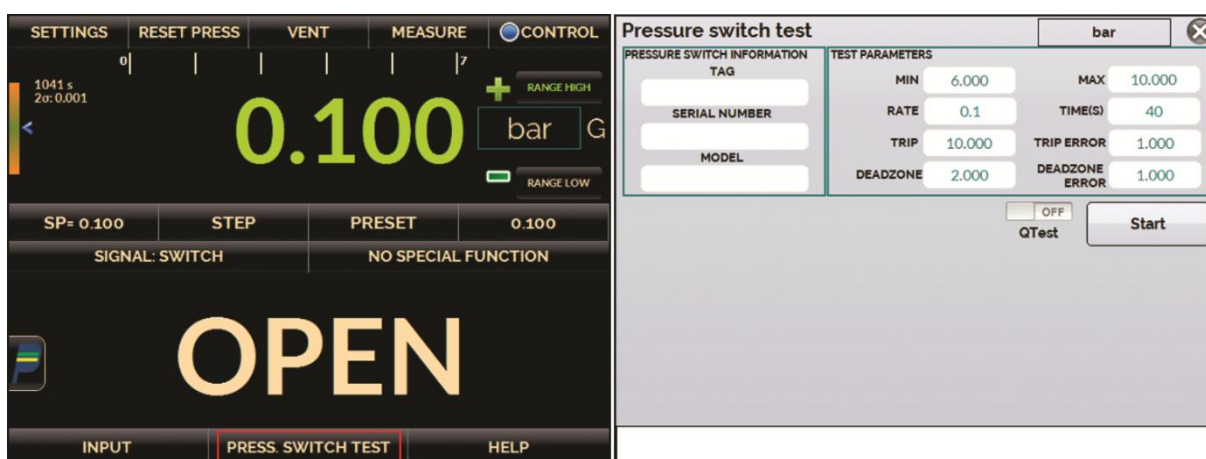
Fig. 48 – Pressure Switch Test 壓力開關測試
