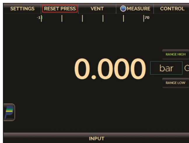
Fig. 32 – Reset of the current pressure measurement. 恢復原來之壓力狀態
