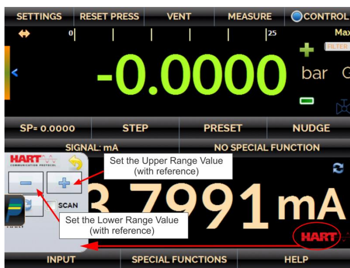
Fig. 63 – Quick HART® Adjustment with Reference. 快速用 HART®來規劃測量範圍
