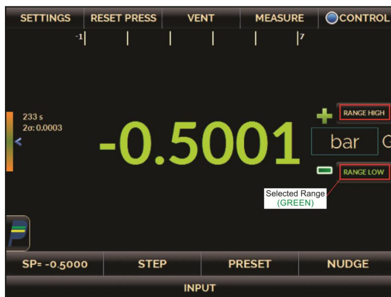
Fig. 16 – Selecting the Pressure Range 選擇壓力範圍
