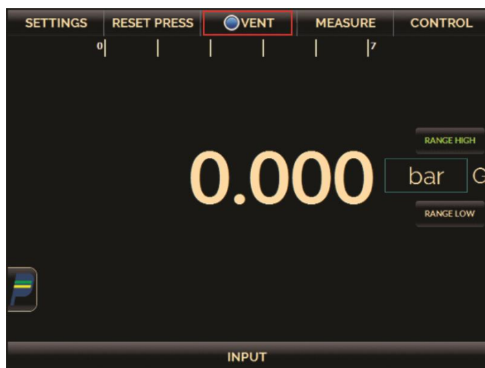
Fig. 30 – VENT mode on the OPERATION screen 畫面之上.
