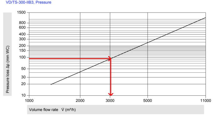
Capacity loads as per PROTEGO Diagrams refer to air as per ISO 6358 at 20°C, 1 bar The capacity curve is measured with a clean flame arrester.
