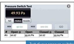
Test of your pressure switches can be performed automatically.
