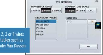
RTD can be connected with 2, 3 or 4 wires and you can select various tables such as the IEC 60751, JIS or Callender Van Dussen
